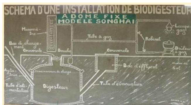
Figure 5: Diagram of a bio digester installation
